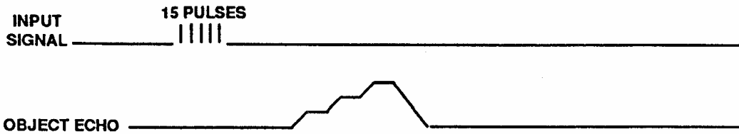
Example of the REC Pin Response to 15 Cycle Burst (test circuit)
