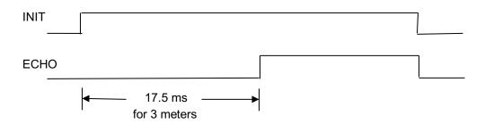
Normal Blanking time = 2.38 ms. When BINH, BLNK are not used, the minimum ECHO return will be 2.38 ms for a minimum target distance of 0.41 meters (16.1 inches) at 20° C.
